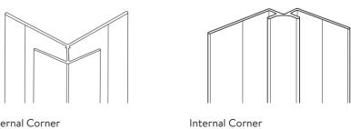
End Cap Use these profiles when needing to join two panels on an internal joint.
